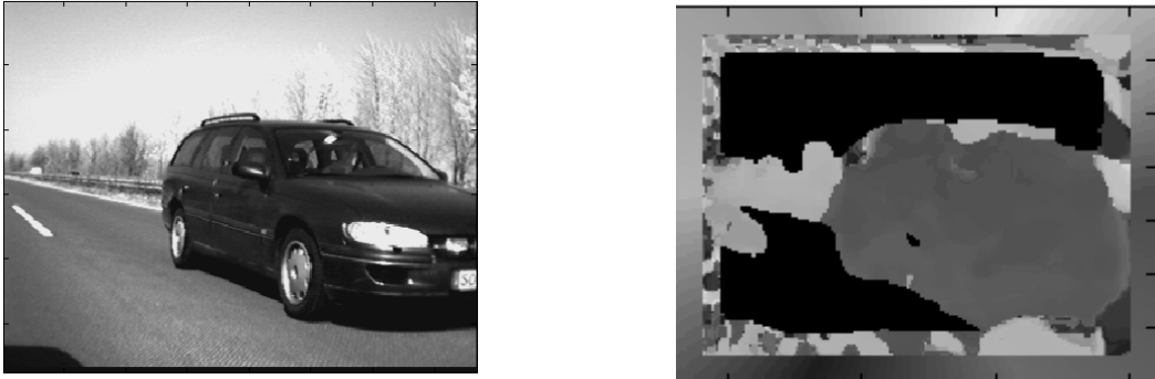
Fig. 4. Car segmentation using optical flow. Dark greys represent rightward movements (the car) and light greys leftward motion (the landscape). We can see that the proposed model gives us a very uniform object segmentation therefore car tracking can be done easily.
