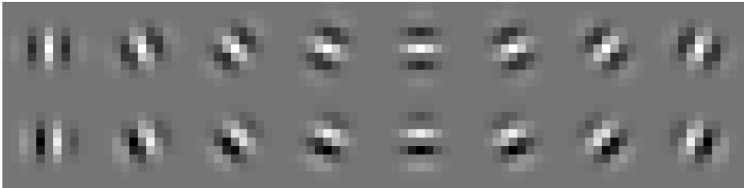
Figure 6. Example 4th order filters for u_{\text{peak}}=1/4 , 8 orientations and using 11 taps are shown below.
