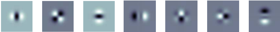
Figure 7. Second order Gaussian derivatives separable base set. The three first filters (from left to right) are the Gaussian derivatives and their Hilbert transforms are the four filters showed on their right. With this set of filters, we can estimate the output at any orientation just combining linearly the base set output. This allows building oriented quadrature filters banks as shows in Figure 2.3 but at any possible orientation.
