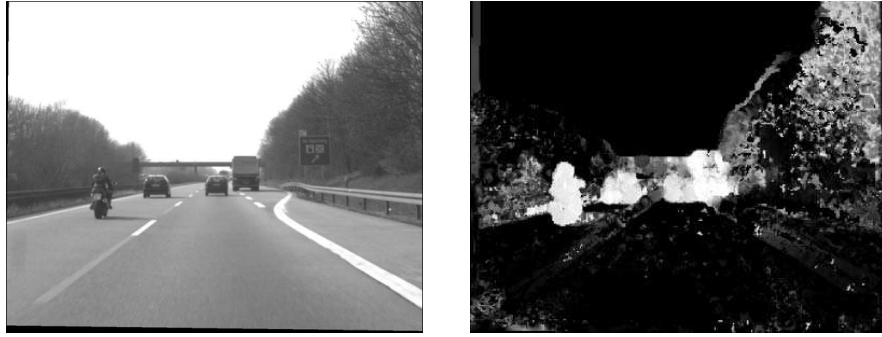
Fig. 5. (Left) Frame number 342 of motorway3 sequence. (Right) Matrix I , output of the motion stream for the same frame. Value I(x, y) is defined as probability of pixel (x, y) being part of an IMO.
