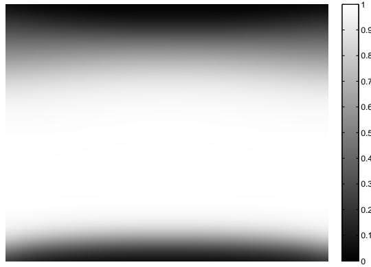
Fig. 9. Matrix M , masking regions of possible IMO appearance in a frame. This matrix has been chosen heuristically based on the logical assumptions that in normal circumstances IMOs are not supposed to appear “in the sky” or beneath the ego-vehicle.
