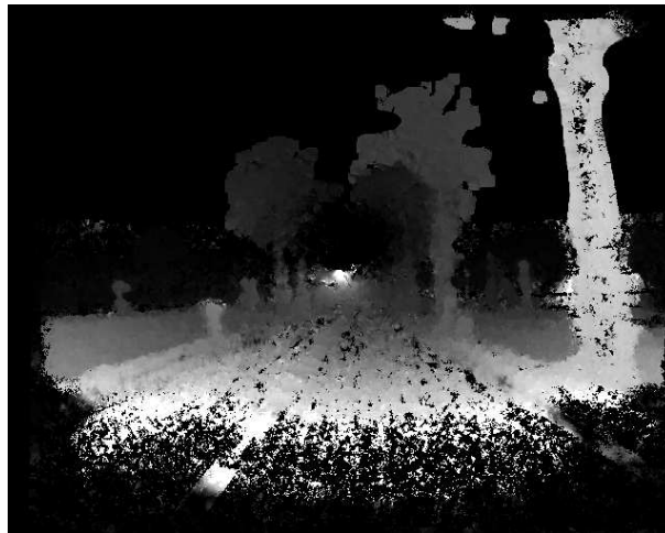
Figure 8: Depth map obtained from the a posteriori estimate of the depth map by using the Kalman Filter update.
