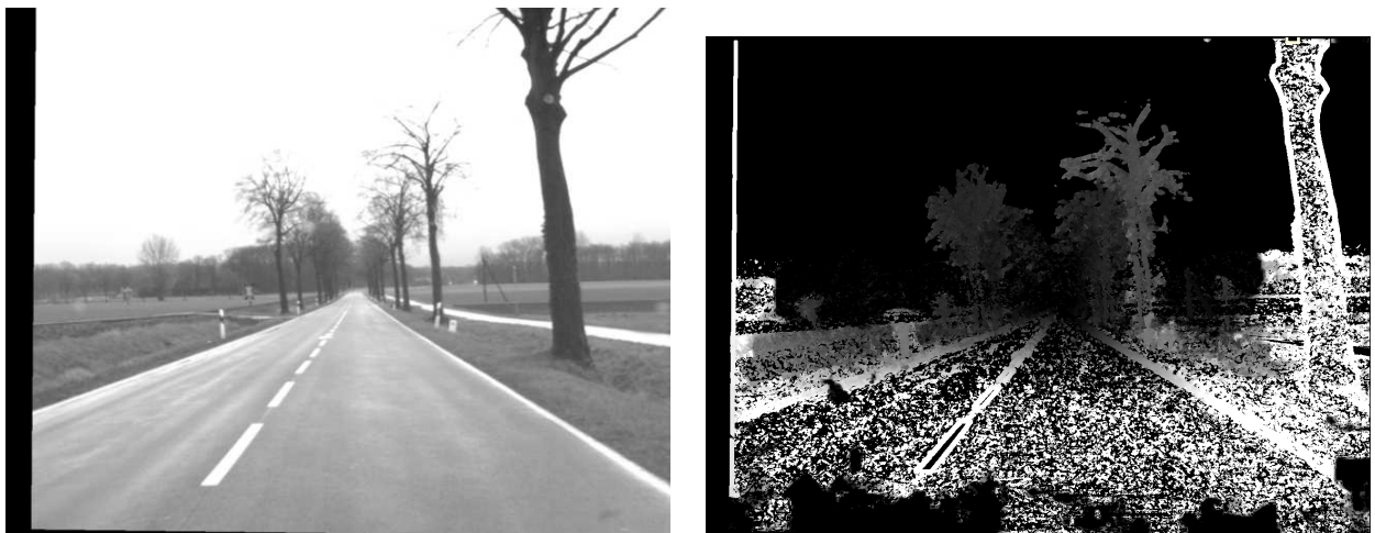
Figure 4: (a) Frame from a street sequence. (b) Depth map obtained with the phase-based algorithm for disparity (using only non-visual cues).
