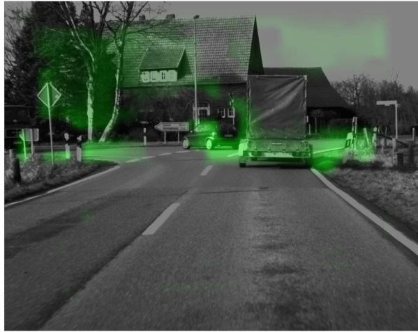
Figure 12: Map representing the time to collision. The truck is moving along the same direction of the observer, and its TTC is higher than the one to the still objects at the same depth
