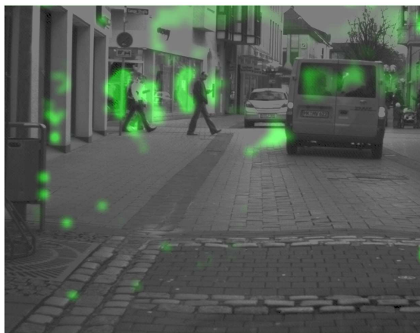
Figure 13: Map representing the time to collision. The van is moving along the same direction of the observer, and its TTC is higher than the one to the still objects at the same depth
