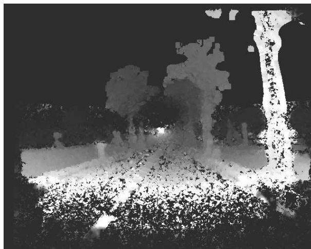
Figure 7: Depth map computed using the non visual signals together with visual information (optic flow), without the Kalman Filter update.
