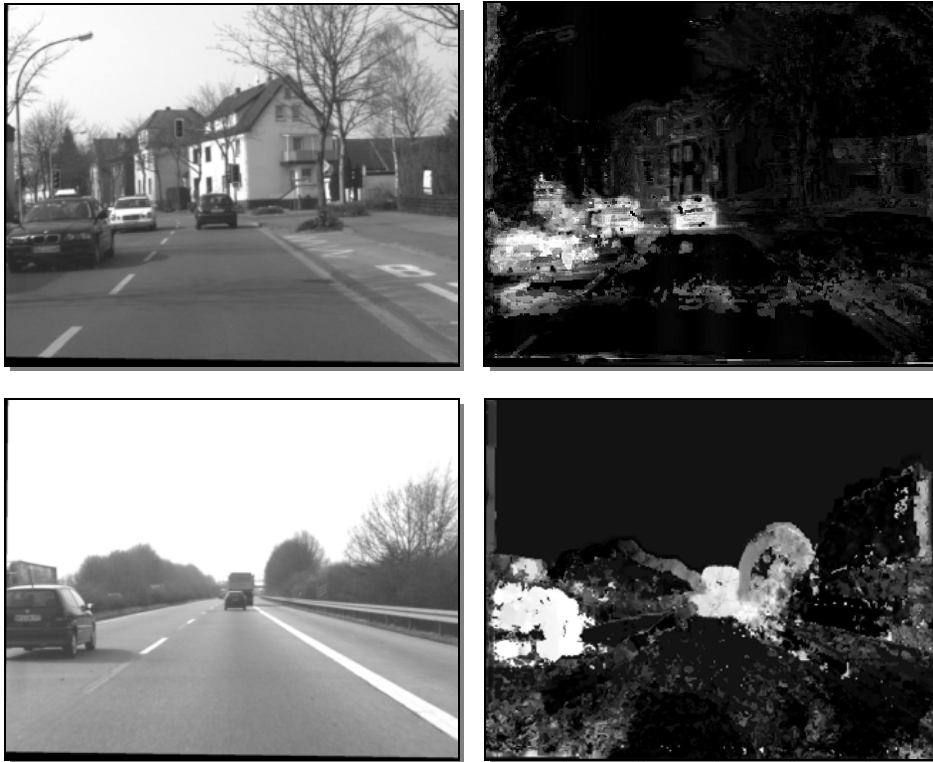
Fig. 1. Left images are rectified versions of original (left) frames taken from sequences city3 (upper) and motoway3 (lower). Right images are independent motion maps corresponding to left images.
