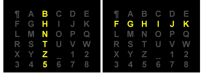
Fig. 4. Typing matrix of the mind-typer. Rows and columns are flashed in random order; one trial consists of flashing all six rows and all six columns. The intensification of the third column (left panel) and the second row (right panel) are shown.
